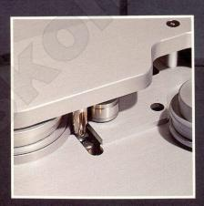
An Optical end of tape sensor is standard on all A80VU recorders. This sensor deactivates the electronic tape timer and initiates the stop mode at the end of the tape.
