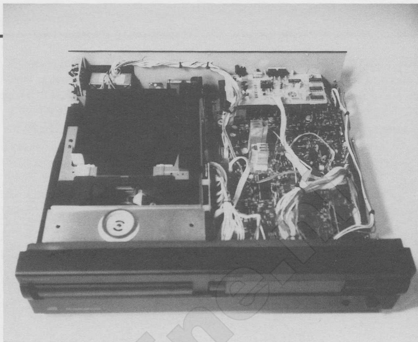
The 1+6 stoker mechanism is located in the upper left corner; at lower left is the large, round disc stabilizer; at upper right, are the dual D/A converters; between the D/A converter and stoker mechanism are the isolated-ground power supplies
