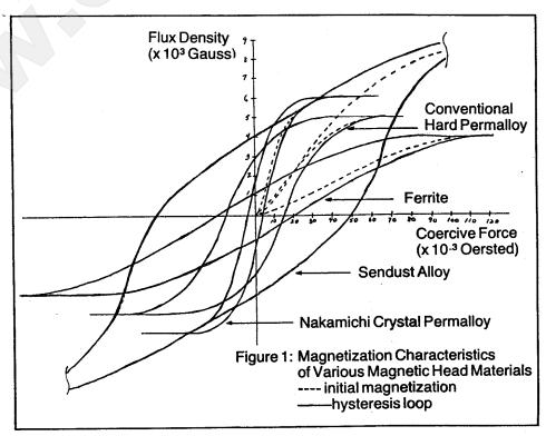
coercivity display rather elongated hysteresis loops and highly non-linear initial magnetization. Nakamichi Crystal Permalloy is characterized by a highly desirable low coercivity. Its hysteresis loop is very vertical; its initial magnetization, as a result, is comparatively linear.
