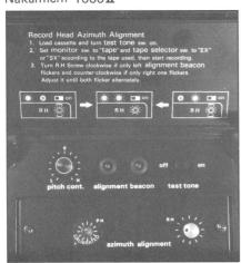
Before recording, please be sure to adjust the record head azimuth using the record head azimuth alignment beacon whenever you change cassette tapes (even when you change from side A to side B of the same cassette tape).
