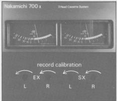
• If the levels are not within 1 dB of "0 dB", adjust the appropriate level calibration controls (Left or Right, EX or SX) clockwise or counter-clockwise (Fig. A or Fig. B) to obtain a 0 dB reading on both meters.
