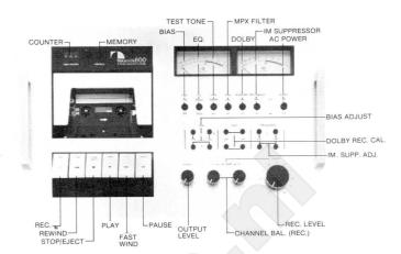
The Equipment: Nakamichi 600, a stereo cassette deck with IM Suppressor and Dolby noise reduction, in metal case.
