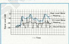
The extraordinary dynamic range of the Nakamichi 550 permits the use of 45 dB peak reading meters. These large full-range meters are exclusive with Nakamichi and have a very fast attack time (120 ms) and a slow release time to more accurately reflect true recording conditions. They are especially helpful in preventing over-recording during live sessions.
