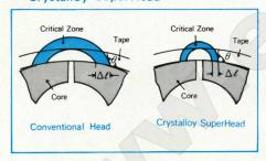
This simplified illustration shows how the record head applies magnetic modulation to the tape during recording.
