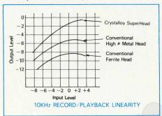
For playback, the head gap should be critically maintained at 1.5 microns or less to assure superior high frequency performance. Unfortunately, with most heads the "effective gap" is extended magnetically (often to 2 microns or more) due to stresses imposed during their manufacture. To avoid this problem and the attendant high frequency losses, Nakamichi has developed advanced micro-precision head assembly techniques that prevent magnetic extension and insure an unvarying gap of 1 micron.
