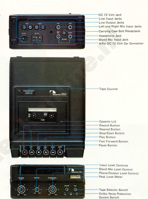
Note: The 350 provides line and headphone outputs only. It has no built-in power amplifier. Its use in car stereo systems, therefore, requires an external 12V power amplifier. Conventional car speakers cannot be connected directly to the 350. The ADS 2001/2002 miniature speaker systems are ideal for use with the 350 since they provide their own bi-amplification.
